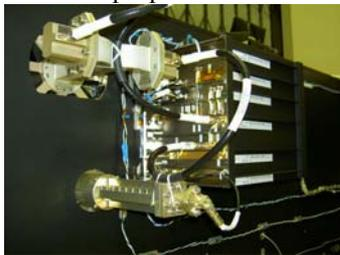
The KaTE experiment will validate new digital communications technology with very sensitive receivers onboard the spacecraft acting as a precursor for future deep space missions. New data encoding techniques enhancing the link performance will also be tested.
