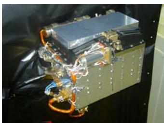
The detector head comprises a matrix of 24 X-ray sensitive Swept Charge Devices, collimators defining field of view and filters blocking background
