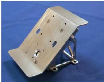
**KaTE** Deep Space X/Ka-band Telemetry and Telecommand Experiment, The experiment is being managed by ESTEC in conjunction with Astrium, Germany.
