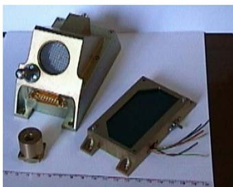
The payload constitutes an electronic unit and a number of sensors positioned on the outer surfaces of the spacecraft. The Plasma probe assembly, located close to the EP motor will monitor the backflow of electrons. A Langmuir probe measures the plasma potential and a Retarding Potential Analyser will measure the ion energy and current density distribution. A solar cell and a
