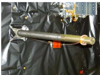
This payload consists of two electric sensors mounted at the ends of 60 cm booms located on the opposite sides of the spacecraft. The sensors, controlled from an electronic unit, can be configured either as Langmuir or Electric Field probes. SPEDE will be used in conjunction with EPDP to monitor the EP motor plasma effects on the spacecraft. In addition the experiment will perform mapping of Earth and Moon plasma density and solar winds coupling to the Moon.
