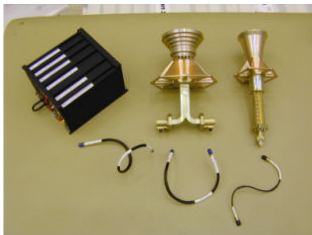
KaTE TRSP with X and Ka band antennas and interconnecting RF cables
