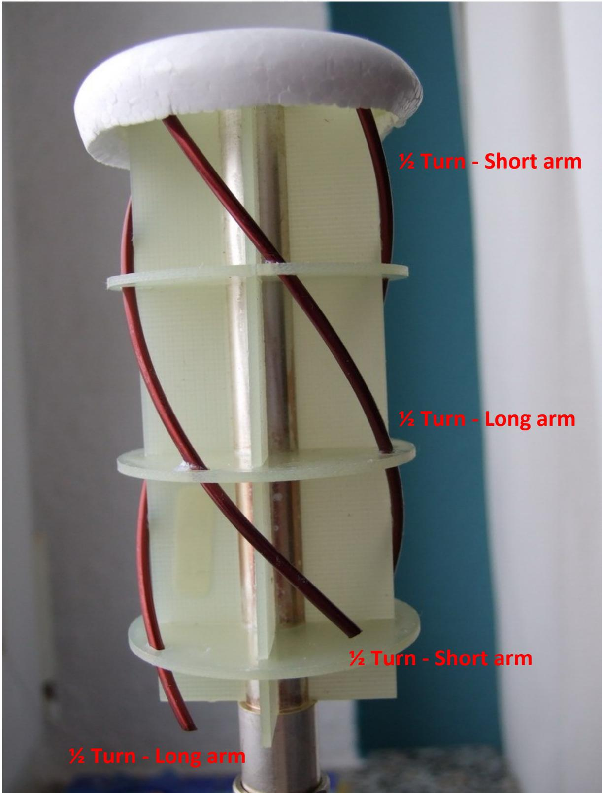
Helix structure is supported by epoxy plates (PCB like material). Given the small size a self-support might be possible in a homebrew project or a more simplified support structure.
