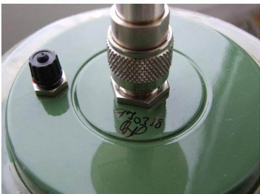
Rubber gaskets are used throughout the construction to make the antenna moisture proof and the electronics compartment of the antenna is backfilled with a dry inert gas via a valve at the time of building to prevent condensation problems occurring by changing environment conditions around the antenna.
