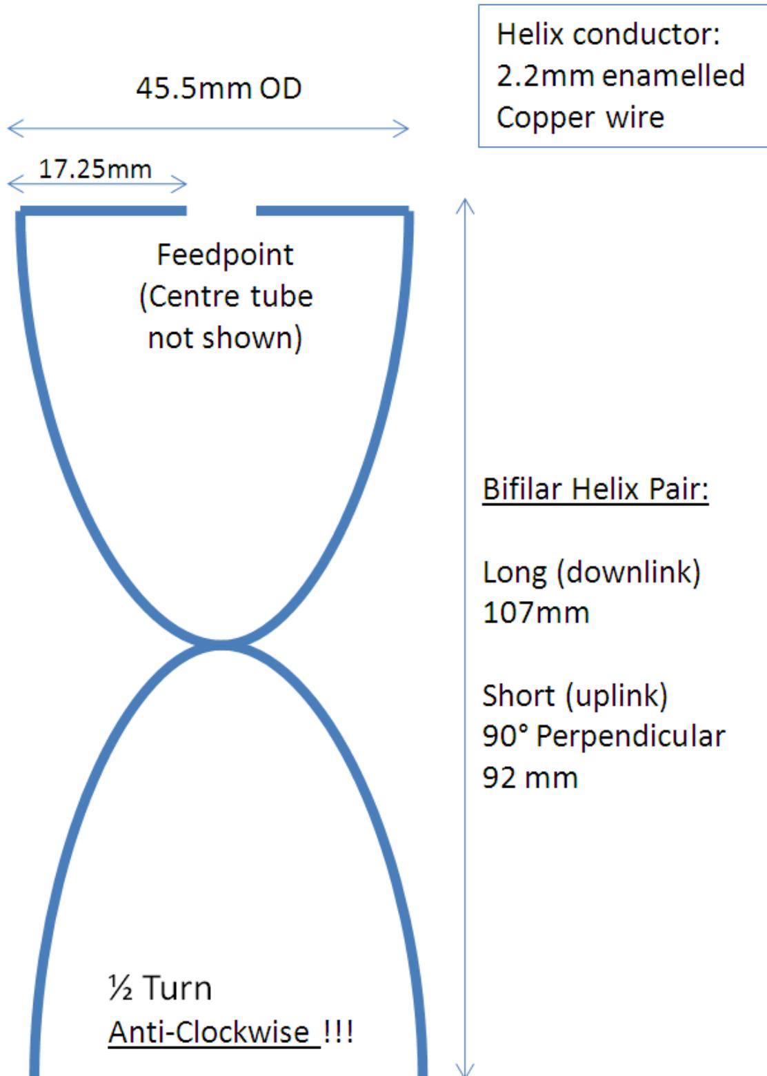
**“Streight” Helix conductor lengths per 1/2 turn arm (before bending into helicoidal shape):**
