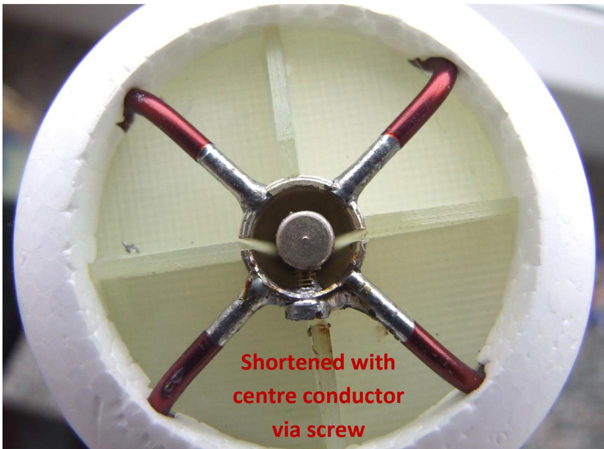
For the construction of the split coaxial line balun it is important to keep the same inner diameter of the central tube till the bottom of the N-Connector case. This means that the tube and the short diameter reduction tube should be pushed all the way down into the N-Connector. The 5mm centre conductor needs to be connected to the centre pin of the N-Connector.
