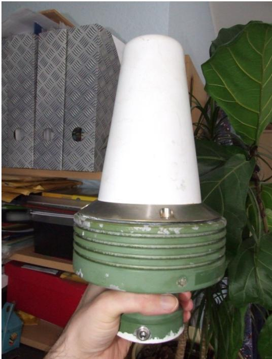
The antenna helix element sits under a plastic radome. The cast metal base is the housing for the built-in electronics (Combiner, Diplexer, Low-Noise RX Preamp and Uplink Power Amplifier). The base also serves as the ground plane for the helix antenna element.
