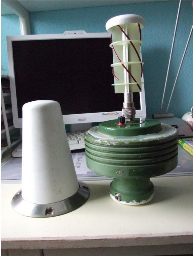
The antenna element itself consists out of a N-Type connector at its bottom followed by a short tube for the purpose of diameter reduction, followed by the main centre tube.
